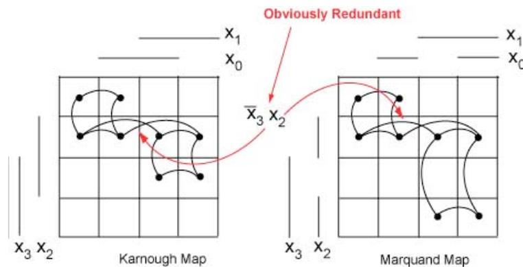
Figure 8-2 Reducing a Simple Function
