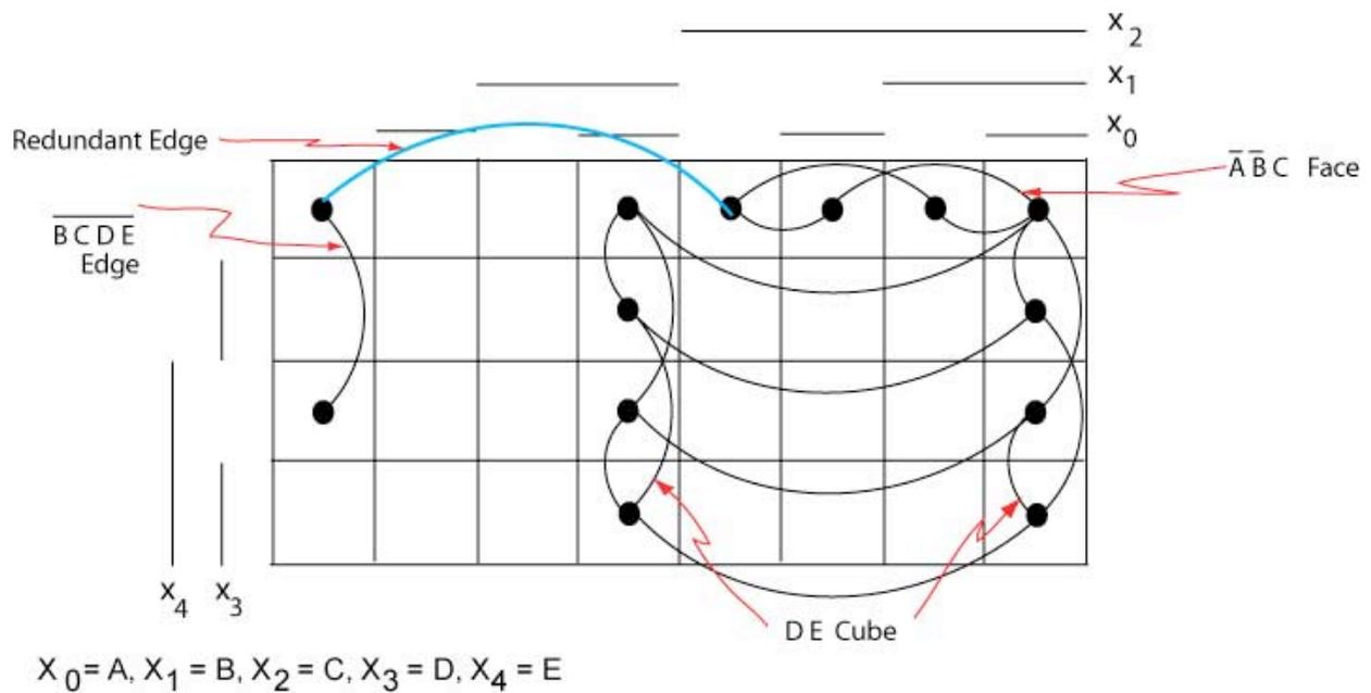
**Figure 8-3 Algebraic and Map Minimization of a 5-Variable Function**
