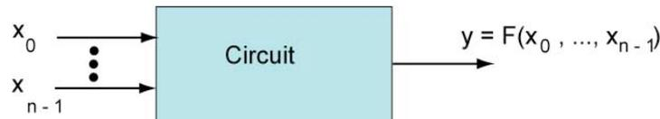
Figure 8-1 Combinational, Single-Output Circuit
